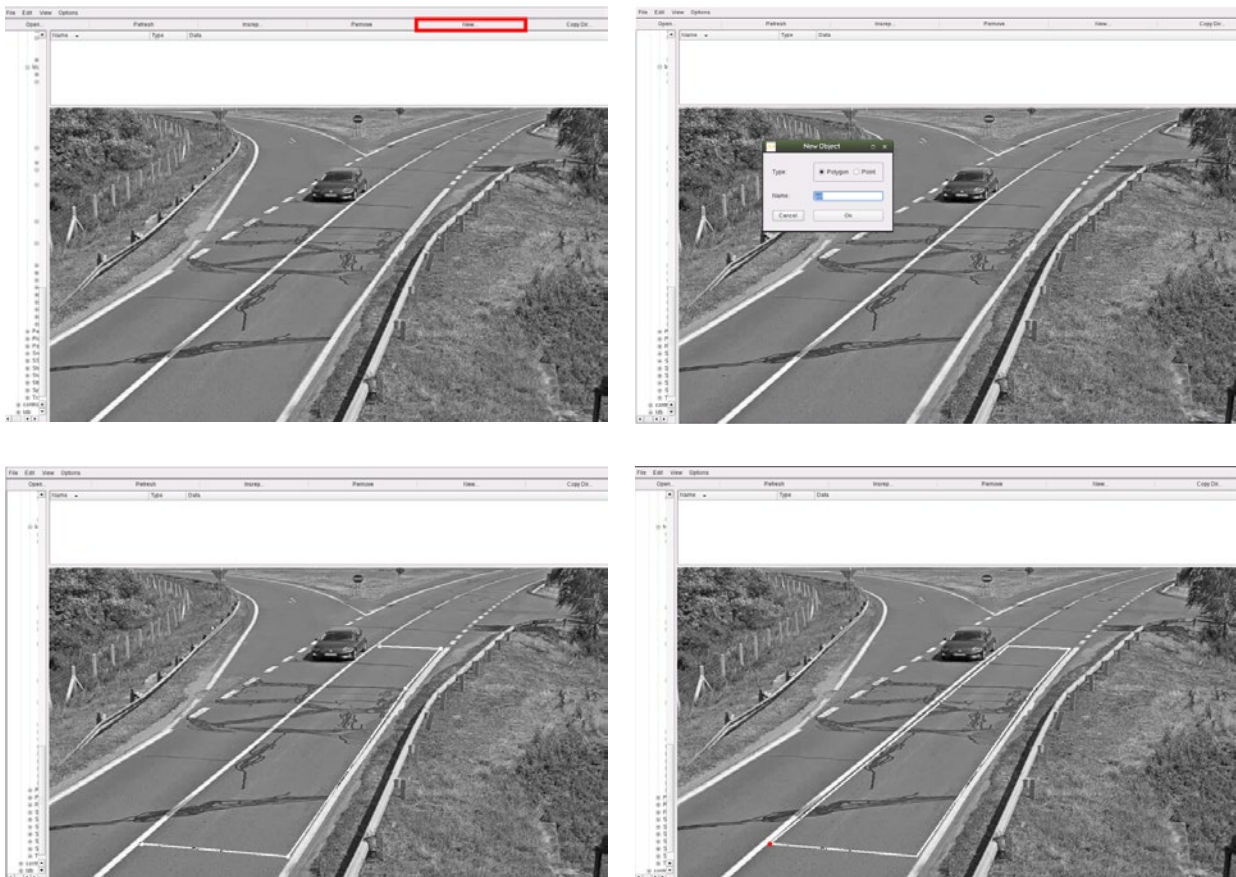
Figure 11: Steps for drawing a new polygon –Creating a new polygon (top left), Setting the name (top right), drawing all sides of the polygon except for the last (bottom left), closing the polygon (bottom right)
