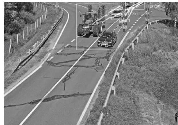
Figure 9: Solid Line Crossing, detected by the sequence 1..0 (left) or using the driving direction evaluation (right)
