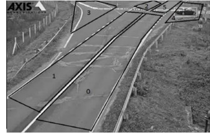
Figure 8: Wrong turn detection, sequence starting with ROI #3 and ending with #4 Incident Detection system
