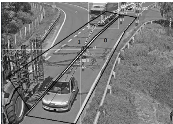
Figure 9: Solid Line Crossing, detected by the sequence 1..0 (left) or using the driving direction evaluation (right)
