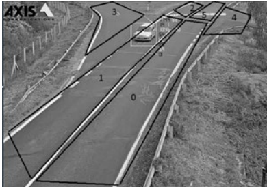
Figure 7: Wrong turn detections- detection based on sequence starting with ROI #4 and ending with ROI #1 (4..1, left), detection based on sequence starting with ROI #0 and ending with ROI #4 (0..4, right)
