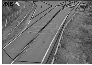
Figure 7: Wrong turn detections- detection based on sequence starting with ROI #4 and ending with ROI #1 (4..1, left), detection based on sequence starting with ROI #0 and ending with ROI #4 (0..4, right)
